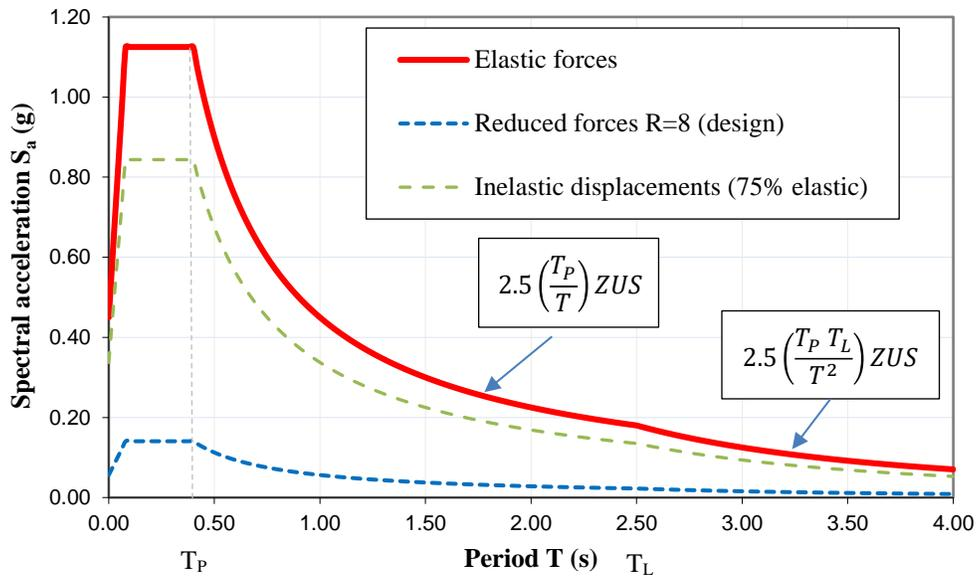
Fig. 1: Seismic Peruvian standard E.030 spectrum – 5% Damping – RC moment frame regular building.
