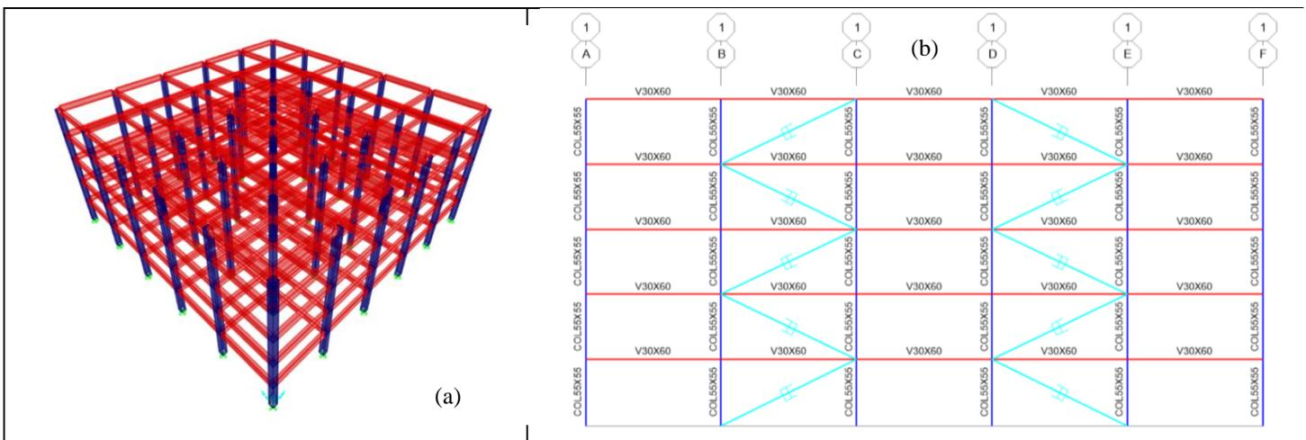
Fig. 2: (a) SAP2000 model of the RC moment frame building and (b) location of fluid viscous dampers.
