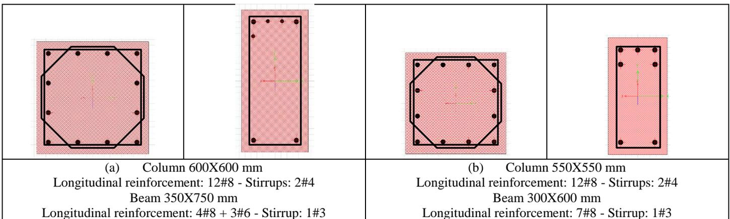
Fig. 3: Typical bars at column base and bars for maximum moment in beams for (a) reference building (b) building with FVD.
