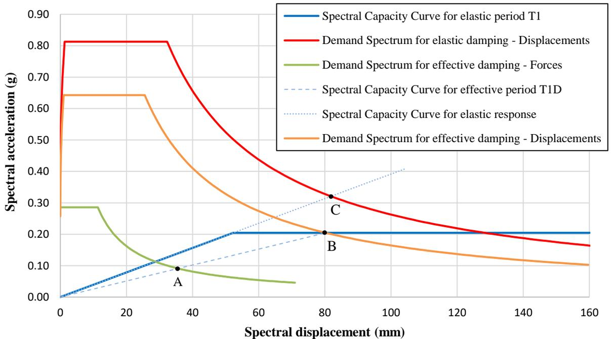
Fig. 4: Response on the fundamental mode – Building with linear FVD – Spectrum of E.030 standard.
